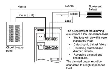
FIG. 3 RDM-2DC application wiring
